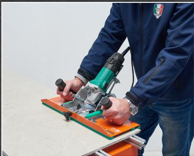
Strong structure, precise and fluid sliding with polyethylene pads, practical and comfortable handles on which to apply the pressure necessary for advancement.
