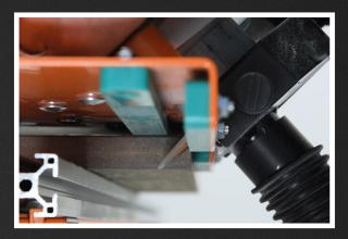
Adjustable bevel depth, with maximum cutting height of 21 mm, disc cover with dust extraction.
