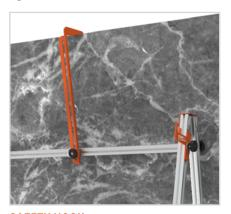
**SAFETY HOOK** Cargo allows you to move one or more slabs using the safety hook to avoid accidental unhooking.
