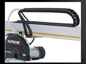
**CABLE CHAIN** The system of the cable chain improves the ergonomics of the machine and its disk water cooling.
